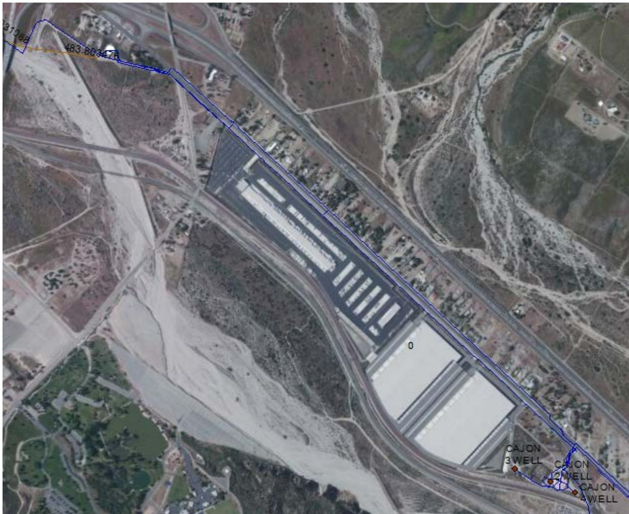
The Kenwood well field is located in Cajon Creek Wash near the Interstate (I-) 215/I-15 junction. The well field is connected to other Water Department infrastructure by an existing pipeline.
